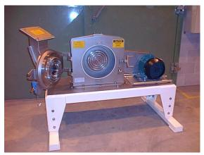
Shown below is a PPS 7CMT mill and the mill's interior, depicting the rotor and classifier, supplied for milling Lactose.
