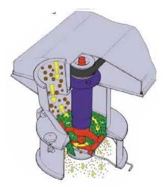
Below is a Kek 680 Cone Mill which increases the Bulk Density of spray-dried Creamer from 28-31 Ibs/ft3 to 37-40 lbs/ft3 before packaging at 8 TPH.
