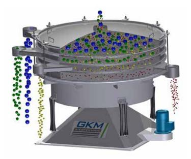
GKM Flat Deck Screening action separates the oversize particles on the top two decks, ideal particles to the third deck and fines to bottom deck
