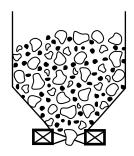
Capable of closing around large particles while preventing the flow of smaller particles.
