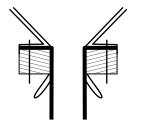
A liner also acting as the gasket between the valve and its mating flange makes a hygienic, easy to clean IBC / valve combination.
