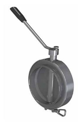
Alternatively, the Clamshell<sup>™</sup> clamp design option can be selected. This enables fast, tool-free strip down and reassembly of the valve in a few seconds. The range consists of 6″ (150mm), 8″ (200mm) and 10″ (250mm) valves which are either manually operated or configured for automatic operation.
